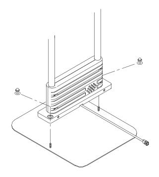
Connect the wire on the power supply to the power wire connected to the antenna. The wires will only connect in one direction.
